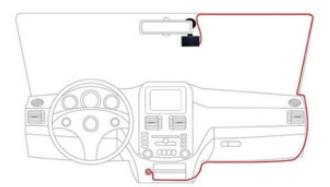
The camera should be positioned near the rear view mirror, in order to have a good front view. The best position is towards the passenger side, as shown, so as not to obstruct the driver's view.
