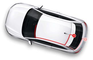
The connection cable is included. On the camera side there is a red cable that you can connect to the positive that turns on the rear lights to automatically bring the rear camera to full screen when reverse gear is engaged. If you don't want this feature you can leave the red cable unused.
