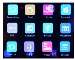
RESOLUTION - Set the recording resolution 1296P, 720P, 480P. Normally the maximum resolution is maintained 1296P corresponding to approximately FullHD, but you can lower the resolution if you want to increase the video archive capacity. Default: 1296P
