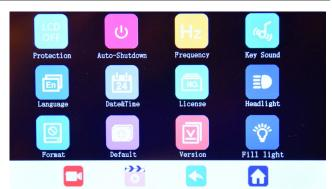
PROTECTION - Activates automatic screen shutdown after 30, 60 or 120 seconds of inactivity. Note that this feature only turns off the screen while the dashcam continues to run. It is very important to enable this function if you keep the camera running while parking to reduce consumption. Default: OFF
